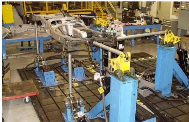
Figure 5-2 Fuel tank strap study setup in test (Photo Courtesy of [36])
